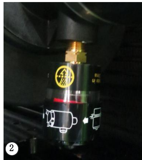
An empty filter Block indicator
