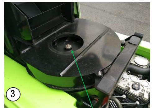
Clean the turbine fan through this opening
