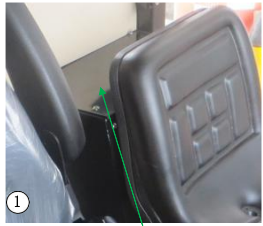
Cover plate of electrical box
