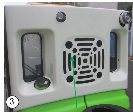
Air conditioning condenser
