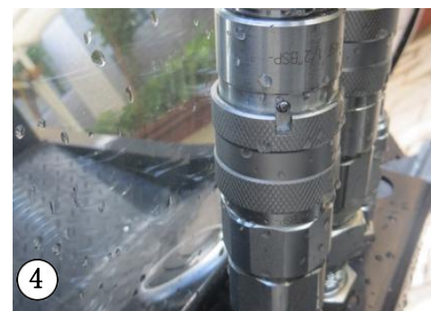
Turn the stop ring to lock the hydraulic quick joint
